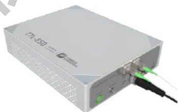
Fig. 1. The compact and miniaturized dual-comb laser device with all optical and electronic parts included.
